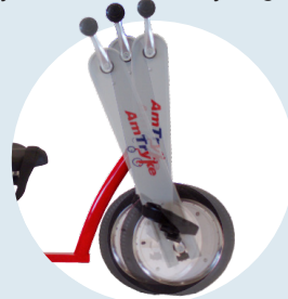
Hinged front end with three positions for adjustable hand crank/foot crank to seat alignment.
